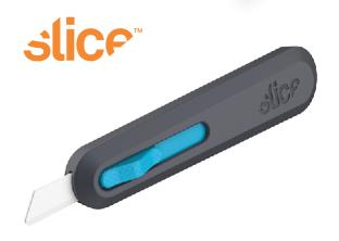
The Slice Smart-Retract Utility Knife combines our patented ceramic blade with the next advance in safety features: smart-retract technology. The Smart-retract feature ensures that the blade retracts as soon as it loses contact with your cutting material, even if you forget to release the blade slider. This protects against slipping accidents because the blade is exposed only when it's doing its job.
